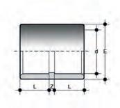
MIC Solvent weld double socket
