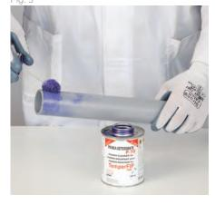
TemperFIP100® or Primer P70 also performs the important role of softening and preparing the surface to receive the solvent cement, an operation that enables a perfect joint to be obtained.
