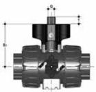
**Power Quick/CE**The valve can be equipped with electric actuators, using the PP-GR module reproducing the drilling pattern foreseen by ISO 5211
