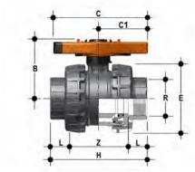
**VXENC**Easyfit 2-way ball valve with female ends, NPT thread
